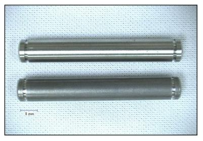
Figure 6 The bottom pin has aluminum oxide residue.
