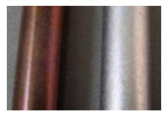
Figure 2 Heat treat scale on left, after mechanical cleaning on right.
