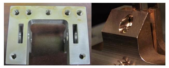
Figure 7 The part on the left appears to have residual chemical run out after processing, the one on the right may have been stored improperly.
