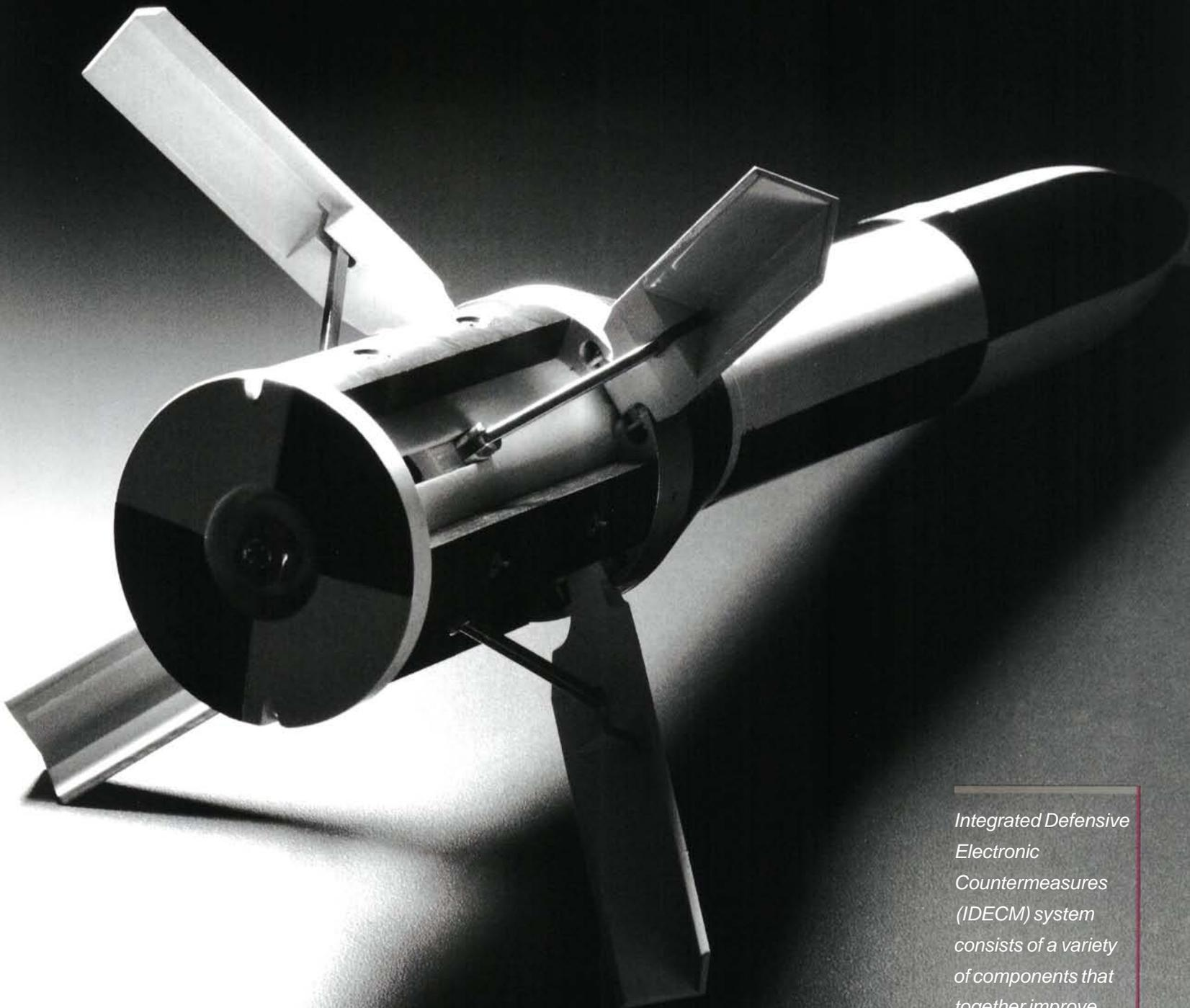
*Integrated Defensive Electronic Countermeasures (IDECM) system consists of a variety of components that together improve the survivability of combat aircraft. The Fiber Optic Towed Decoy, here, is used to confuse enemy missiles.*
